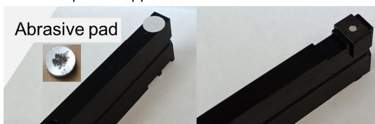
Figure 2: DRIFT sample holders. Left: abrasive pad, right: microbeaker. Inset shows powder applied to the abrasive pad. The micro beaker is shown with powders of \text{MoS}_2 mixed with Csl as matrix material.
