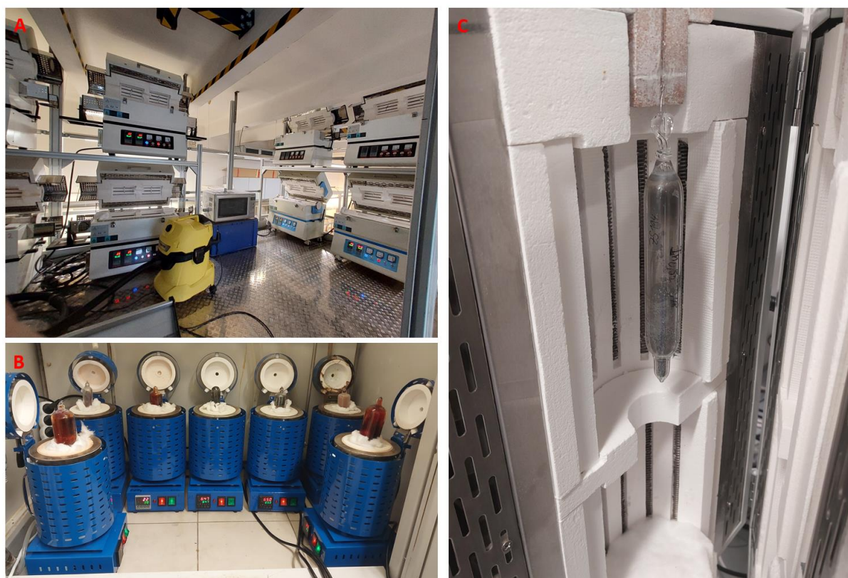
Figure 1. Furnace configurations used for crystal growth: (A) Two-zone CVT furnaces; (B) Crucible furnaces for volatile precursor pre-reaction; (C) Bridgman furnace for melt growth.
