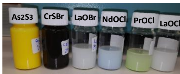
Figure 5. Examples of novel 2D material inks. The inks are in IPA and produced by sonication-assisted LPE from novel 2D bulk counterparts.
